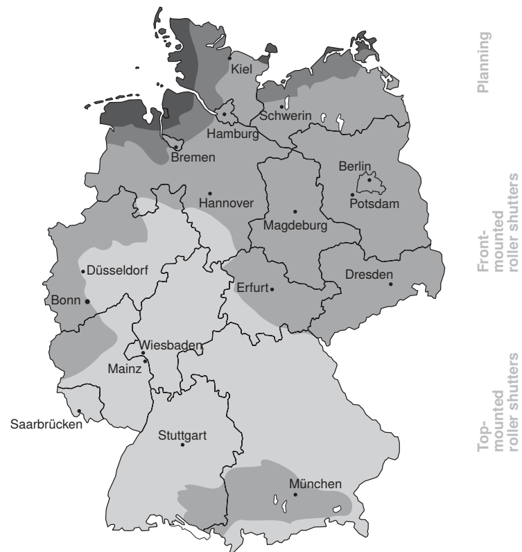
Wind load zones in Germany, Source: DIN 1055-4;2005-03
